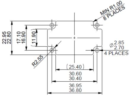
Curtiss Wright recommend the use of  $4 \times EJOT$  WN1451-K25-12 screws when utilising the 4 corner screw mounting points. The screws should be tightened to 0.3Nm with a minimum panel thickness of 3 mm. For thicker panels the screw length should be increased to suit.
