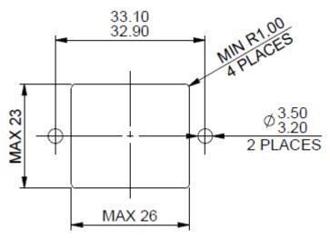
Curtiss Wright recommend the use of 2 x EJOT WN1451-K30-8 screws when utilising the 2 screw mounting points on the centre line. The screws should be tightened to 0.55Nm with a minimum panel thickness of 3 mm. For thicker panels the screw length should be increased to suit.
