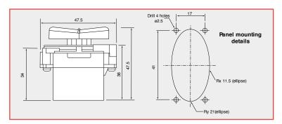
The recommended panel thickness is 3mm. The O ring supplied must be used to seal the JC030 rocker assembly to the mounting panel to enable IP60 protection. Supplied with 4 x panhead Pozidrive self tapping screws for mounting to panel.
