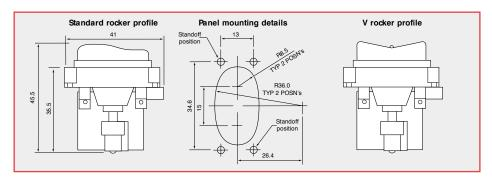
The recommended panel thickness is 3mm. The O ring supplied must be used to seal the JC025 rocker assembly to the mounting panel to enable IP65 protection.
